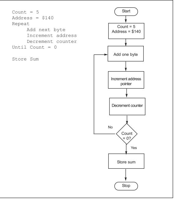
Figure D-7. Pseudocode versus Flowchart for Program D-1
