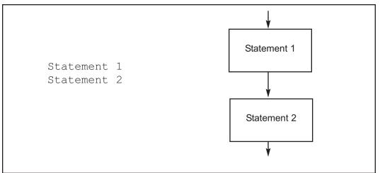
Figure D-2. SEQUENCE Pseudocode versus Flowchart
