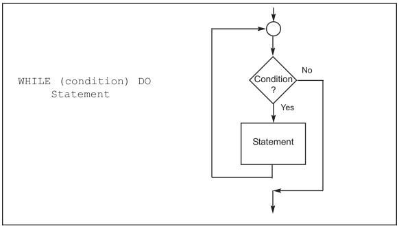
Figure D-6. WHILE DO Pseudocode versus Flowchart
