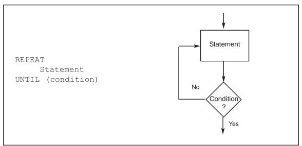
Figure D-5. REPEAT UNTIL Pseudocode versus Flowchart
